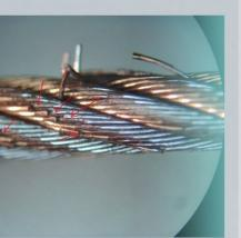
Within the available discard criteria of wire rope due to broken wires (see www.neptunehyrope.com ) these wire ends shall be removed carefully. Best to bend the broken wire end forward and backward until it breaks. Then make sure that the wire ends hide as deep as possible in the gap between the outer strands. Broken wires that stick out of the ropes' surface destroy both the rope and the drum or sheave grooves when running over sheaves and drum.
